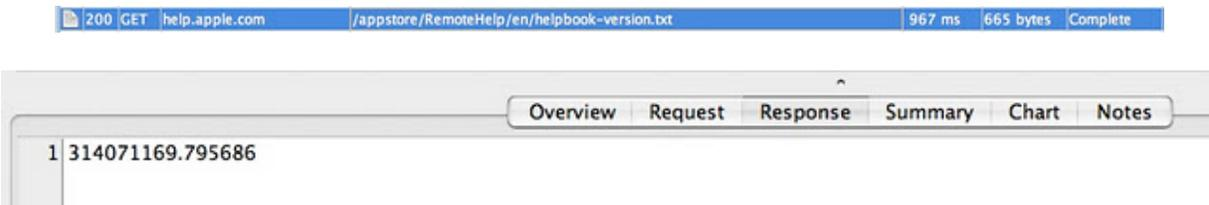
By intercepting this request and serving a different version string, it is possible to trigger an auto update. This was tested using Charles Proxy to simulate the MITM in action by mapping the help book version request to serve a local file with a different version in it:
