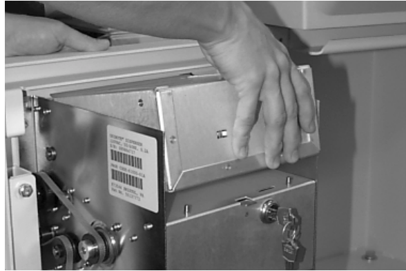
Figure 4-2. Lift cassette to clear the alignment pins.
