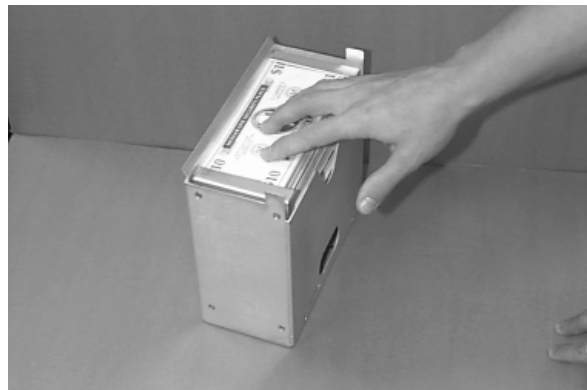
Figure 4-6. Press note bundle into cassette.
