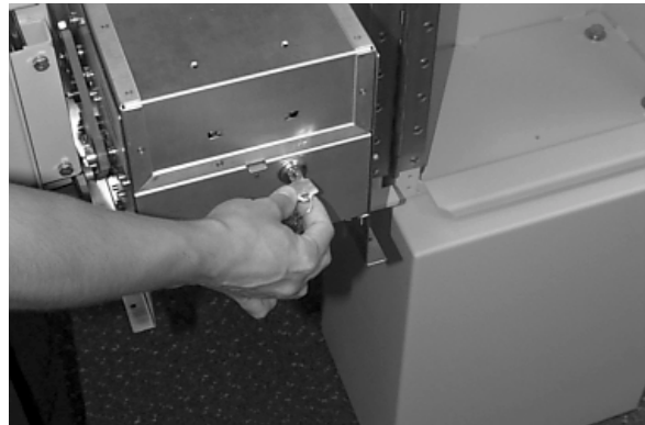
Figure 4-9. Lock the cassette into the dispenser chassis..
