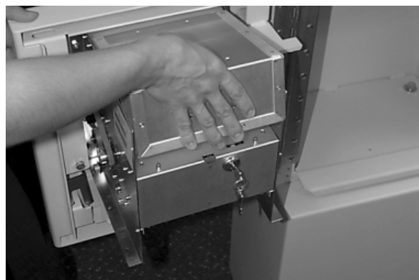
Figure 4-7. Slide/lower the cassette back into the dispenser chassis.
