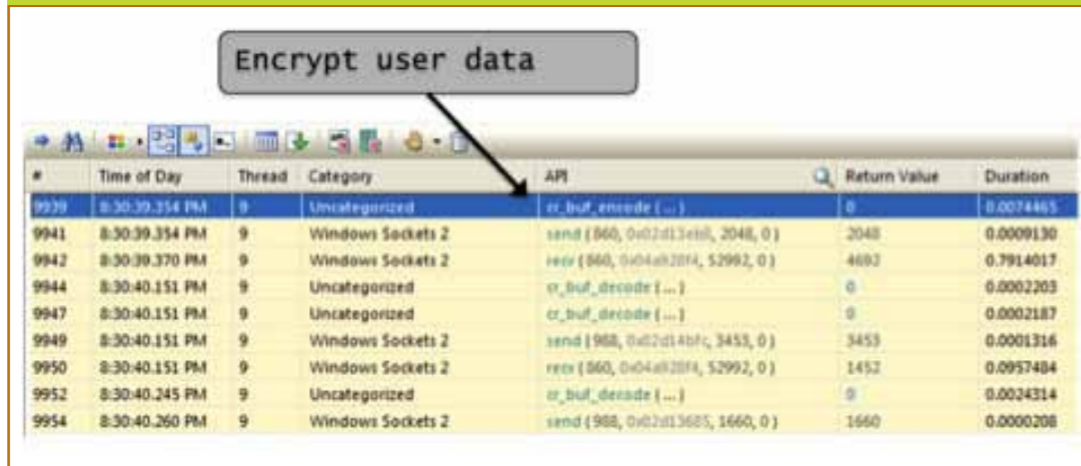
FIGURE 4: A closer look at client trace via API Monitor
