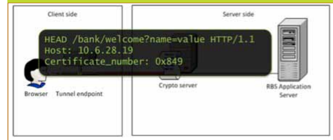
FIGURE 7: HEAD requests pass without signing and checks, crypto client only adds certificate number
