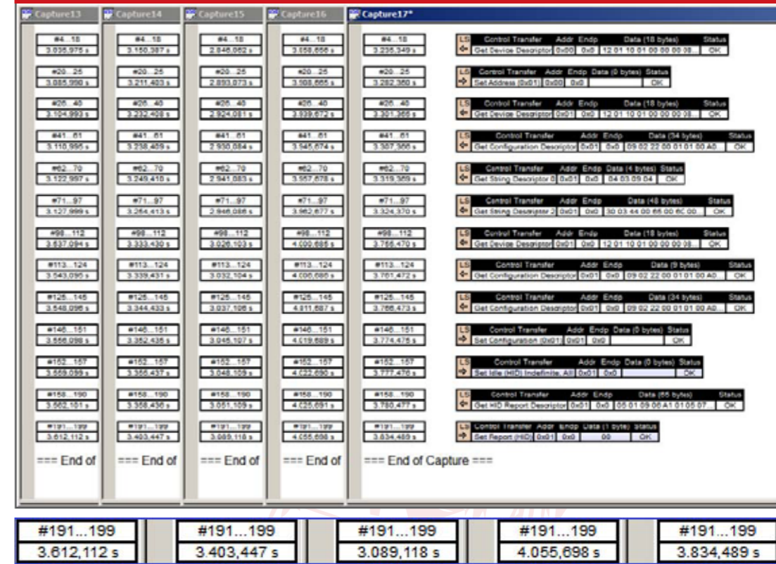
Figure 9: USB timing information during enumeration
