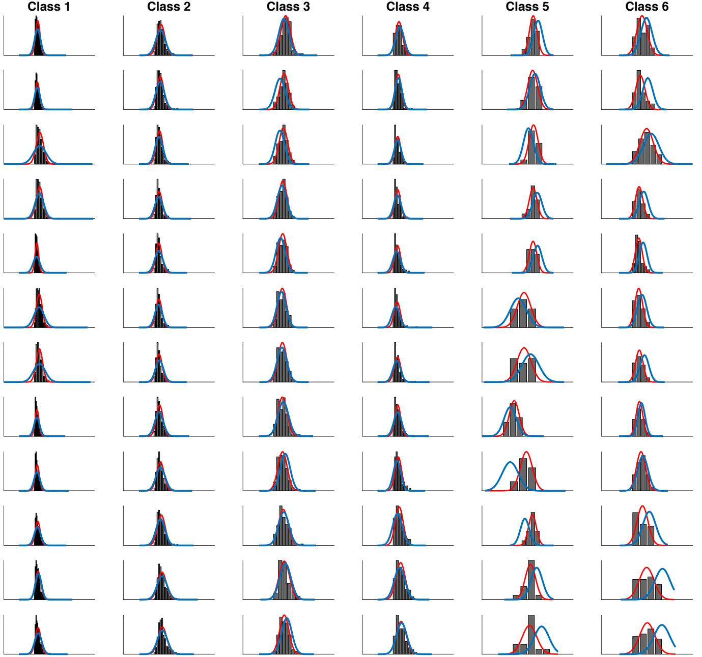
Fig. 8: Entry-wise marginal probability density of GMMs fitted to the AMI load profile data for each class. The subplots in each column correspond to the marginal density of one class. In these plots, the gray bars represent the empirical histograms of the true values, the blue curves represent the marginal density of the GMM computed using the proposed DP method, and the red curves represent the marginal density of the non-private GMMs computed using (2).
