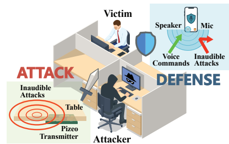
Fig. 1. SUAD: (1) Attack: A piezo-transmitter covertly placed beneath a table emits inaudible signals to attack VAs. (2) Defense: Inaudible perturbation signals block such attacks without interfering with normal voice commands.
