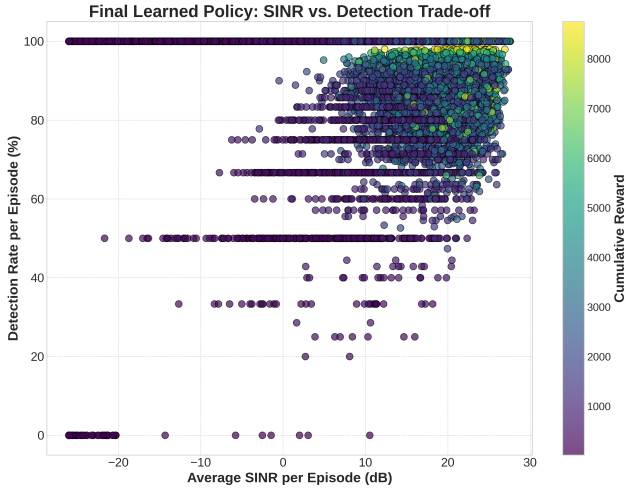
Fig. 3. A scatter plot visualizing the final learned policy. Each point represents an episode, showing the trade-off between the achieved SINR and detection rate, with color indicating the total reward.
