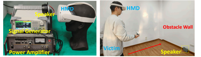
(a) Ultrasonic transmitter system (b) Attack scene Figure 8. Illustration of experiment setup and attack scene. (a) Setup of sound-based trajectory-tempering attack. (b) Attack scene of trajectory-tempering.
