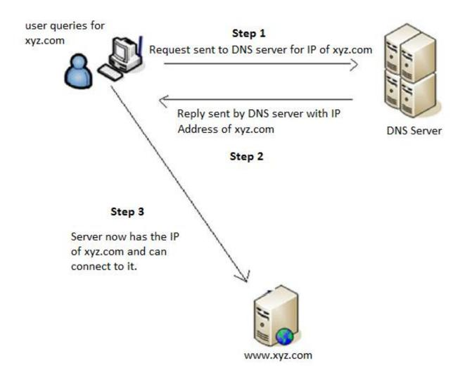
By default DNS works on port number 53 on TCP (Transmission Control Protocol) and UDP (user Datagram Protocol).
