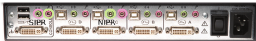
Figure 2. KVM (Avocent, p. 1) configuration example that exploits covert channel using colored circles to show respective jacks to use
