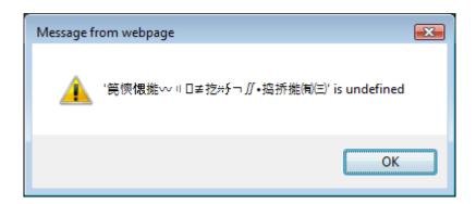
The reason why you see the garbled text is that the JSON bytes are decoded as UTF-16 by the browser, since the SCRIPT element has charset="UTF-16BE" attribute. The decoding process is shown in the table below:
